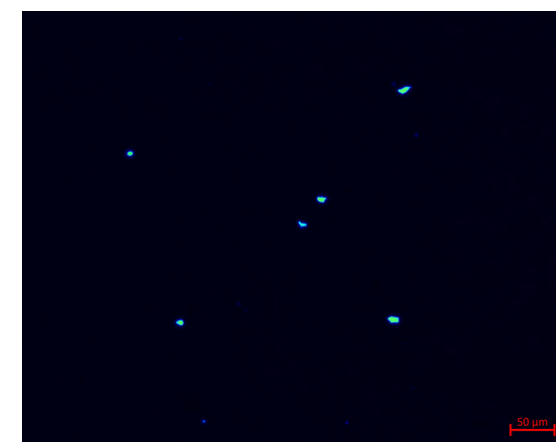
Figure 3: Fluorescence imaging of synthesized carbon quantum dots (x200 magnification).
